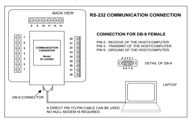
Figure 4.1: RS-232C Communication Connection Installation
